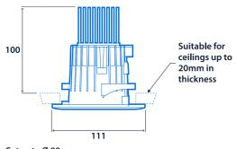
Cut out - Ø 89 Minimum void depth for emergency and AutoTest versions - 165
