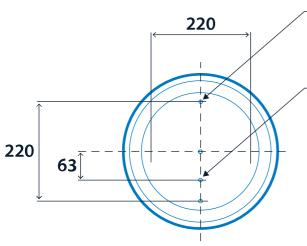
Recommended fixings - 4 x spot faces, drill as required
