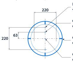
Recommended fixings - 4 x spot faces, drill as required
